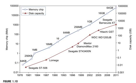
Improvement in memory and disk technologies over 33 years. The Seagate Barracuda XT disk has a capacity of 3 TB in 2011.
