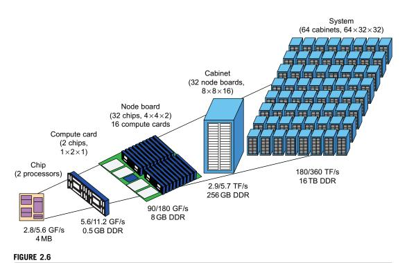
The IBM Blue Gene/L architecture built with modular components packaged hierarchically in five levels.
