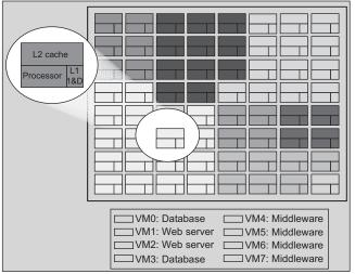
(a) Mapping of VMs into adjacent cores
